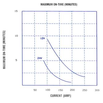
Notes: The thermal characteristics of percent on-time and maximum on-time of the standard duty and medium duty motors are identical. The medium duty motors are UL listed and do offer extended brush life over the standard duty motors.
