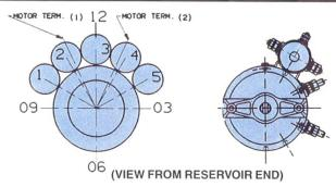
The view above shows start switch locations 1-5 as they relate to motor terminal location "12" only. An alternate example at right shows one of numerous motor terminal and start switch location possibilities that are available.
